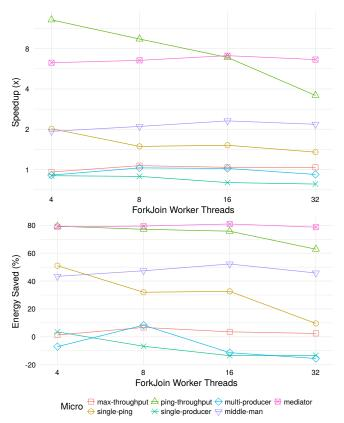
Fig. 1. Speedup (Y-Axis in Logarithmic Scale) and Energy Saving of Refactored AKKA Implementation
