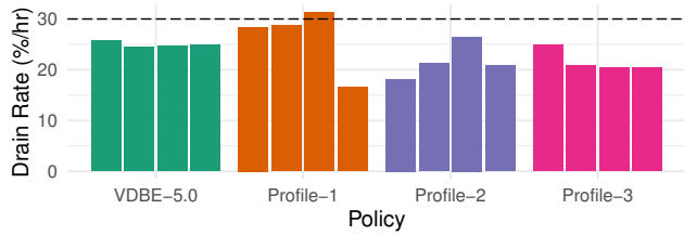
Figure 6: Stochastic vs Non-Stochastic Approaches: Each bar represents a single drive that lasts for approximately 1 hour (120 interactions). The Y-Axis shows the percent battery drain rate per hour of the run. The dotted horizontal bar represents the targeted 30%/hr SLA.
